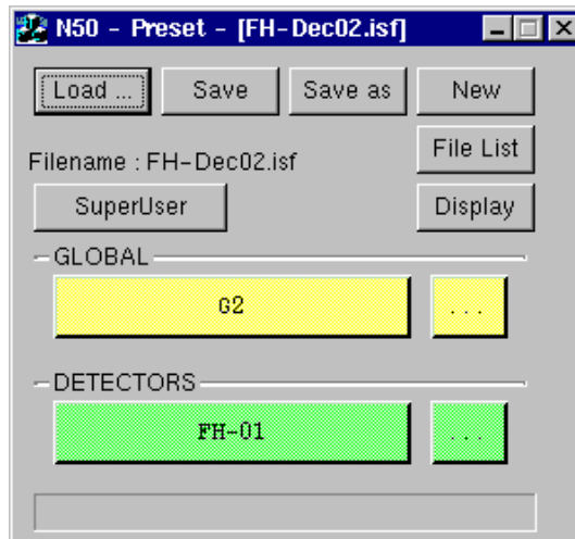
Figure 5-1: The Main Panel of the Preset Menu. In this window the top bar must be blue in order to type in it.
